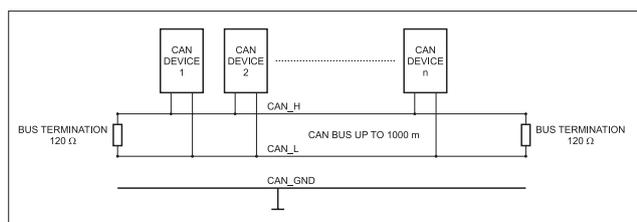
appliances included. In general, it does not matter whether a participant on the bus is a power amplifier or a UCC1 USB-CAN converter, so that both – UCC1 and the PC as well – can be inserted at any position. Incorporating several UCC1 and PCs on a single CAN-bus is also possible. A total of up to 100 appliances can be operated on a single CAN-bus. Since the CAN-
